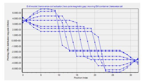
The cross-legs (across the gap) of the coil winding occupy the left and right ends of the plot where the curves are sloped. The magnetic field produced by the current in the coil changes the baseline magnetic flux produced by the permanent magnets alone. That baseline mangnetic flux can be seen in the middle curve which corresponds to the time of zero electrical current. Baseline magnetic flux goes from a positive to a negative value across the gap separating the oppositely polarized magnets.
