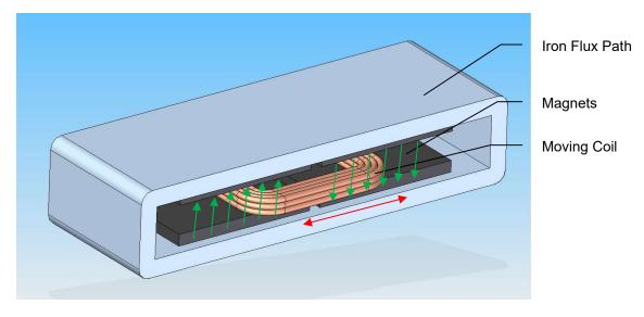
The structure that actually moves and aligns the coil is not shown. In hard-drive practice the coil moves along an arc rather than a straight line and the magnets and iron structure are curved accordingly.
