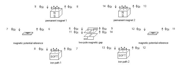
There are two magnetic flow paths laid out similarly to the way they are laid out in the physical actuator, one on the left and one on the right. But the magnets on opposite pole faces (across the gap) are combined together into single magnets. *Permanent magnet 1* representing the left half of the air gap in the above drawing is polarized one way. Permanent magnet 2 is polarized the other way by setting the polarization multiplier input Jmult to -1 in the component *permanent magnet object 2*.
