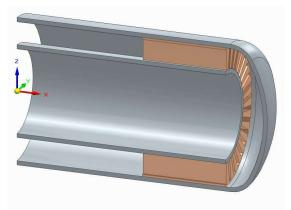
More-or-less following the above rendering, the Sage model consists of a *rectangular fins* component renamed *Pwall to internal fins*, inside of which are two *distributed conductors* renamed *pressure wall* and *outer conductive ring and* a *conductive surface* renamed *fin path*. An *independent line heat source* anchors the pressure wall outer temperature:
