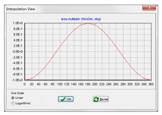
Viewed under the view interpolation option of the input dialog the open area multiplier as a function of time looked like this:
