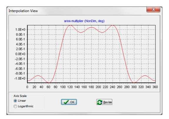
Now the valve opening is more abrupt, although a bit wiggly as a result of truncating the square-wave Fourier series at the 5<sup>th</sup> harmonic. Again, only the values above 1.0E-3 matter. So the valve abruptly opens at 90 degrees and abruptly closes at 270 degrees.
